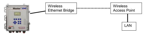
The second solution requires the WM or WA to plug into a wireless Ethernet bridge using a straight-through Ethernet cable, and then the wireless Ethernet bridge connects to a second wireless Ethernet bridge that is plugged into a LAN jack. Two wireless Ethernet bridges are required here.
